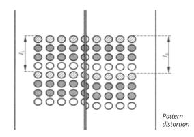
The tolerances for pattern distortion are as follows:
